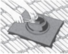
2. Slide down pipe using water as a lubricant, if needed.
