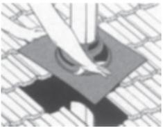
3. Fold 5-10mm of the top of the flashing base up over itself creating a dam and affix under the upstream tile.
